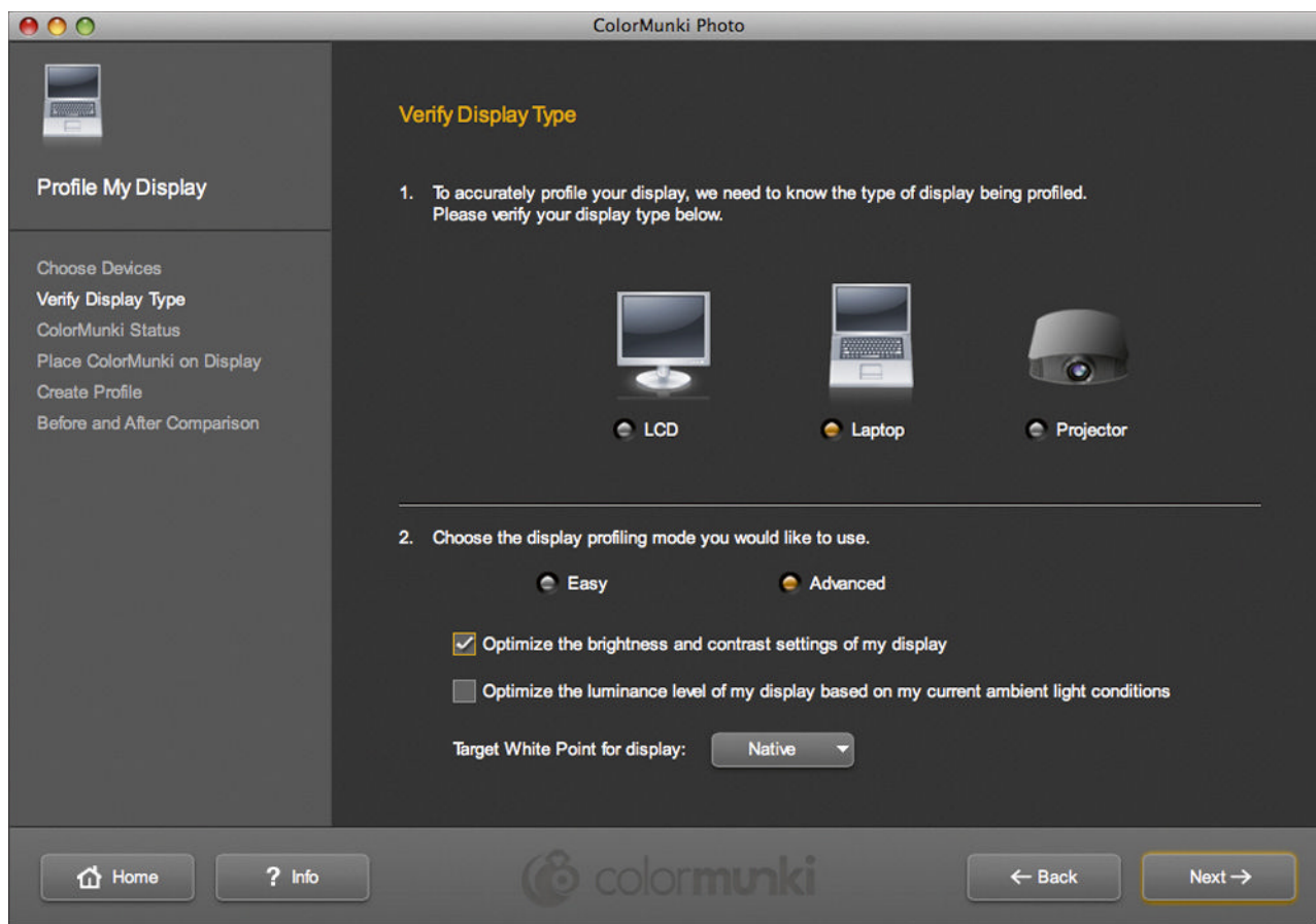
Profiling a display with ColorMunki. The advanced options allow you to optimize brightness and use the native white point of the display.
